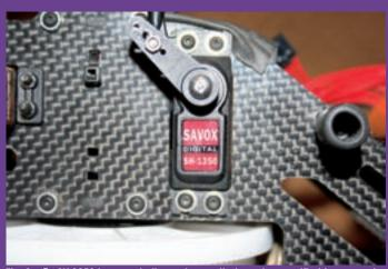
The Savöx SH-1350 is a good all round servo that can be specified for a popu mid-size model like the T-Rex 500 for the CCPM and tail. See table for details
